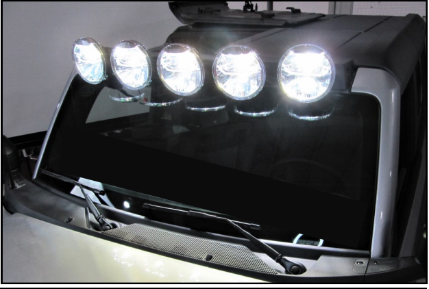
40. Reconnect the Negative battery terminal and perform a function check. With the vehicle running or in accessory mode, the driving lights will be illuminated. With the engine running and the number one overhead accessory switch selected, the projecting lights will be illuminated.
