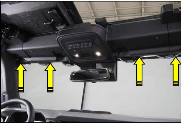
43. Reinstall the trim panels and check for any untucked wiring.
