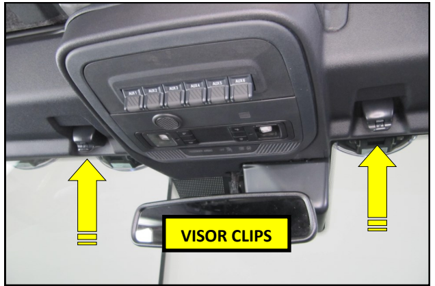
44. Reinstall the visor clips removed in step 7. Do not over tighten.
