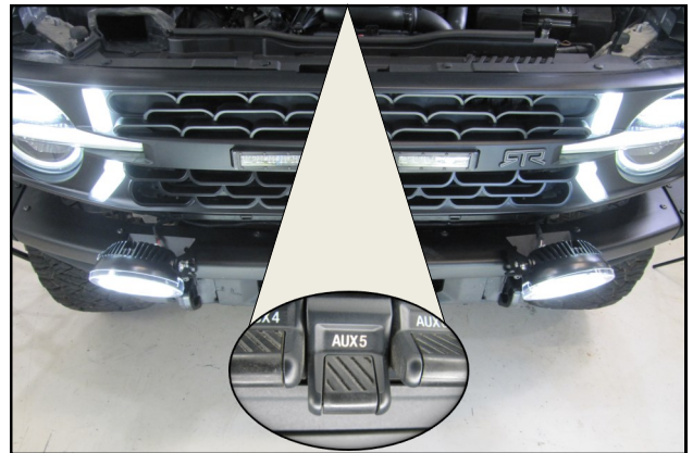
40. Perform a function check: With the vehicle running or in accessory mode, the DRLs in the Auxiliary lights will be illuminated. With the engine running and the number 5 overhead accessory switch selected, the projecting lights will be illuminated. If not, recheck all electrical connections and fuses.
