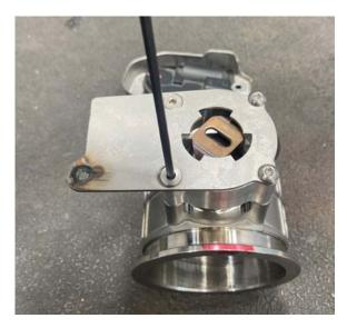
**Step 6:** Once the Clocking Spring is installed reassemble the valve in the order it was disassembled. Take note that the machined spacers have two countersunk holes and they must correspond with the countersunk holes in the plate and the flat head machine screws.
