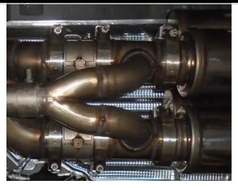
**Step 11:** Next install the Y-Bypass assembly using the supplied 3.00" V-Band clampshe valves using the supplied clamps and fit the electrical plugs.
