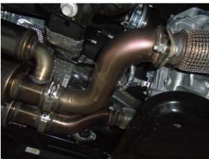
**Step 9:** Begin installation of the MagnaFlow system by attaching the inlet pipe assemblies using the OE fasteners and fitting the hangers into the rubber insulators.
