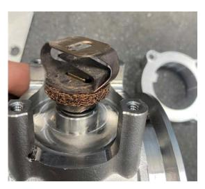
**Step 5:** The valves are supplied assembled, it is necessary to remove the top plate to perform the next step. Remove the Clocking Spring (heatsink) from the OE assembly and install it onto the MagnaFlow valve as shown.
