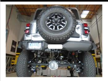
**Step 16:** Once a final position has been chosen for the new exhaust system, evenly tighten all clamps and fasteneners, from front to rear, using the torque specifications on page one of the instructions. Inspect all fasteners after 25-50 miles of operation and re-tighten if necessary.
