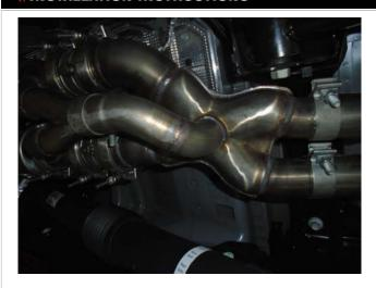
**Step 13:** loosely Fit the X-Pipe Assembly using the supplied 3.00" clamps and fitting the bypass pipe to the Mid Pipe Bypass Pipes using the supplied 2.00" clamps.
