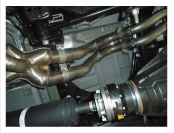
**Step 14:** Attach the Driver and Passenger side over axle assemblies to the X-Pipe using the supplied 2.50" Torca clamps and fitting the hanger into rubber insulator.
