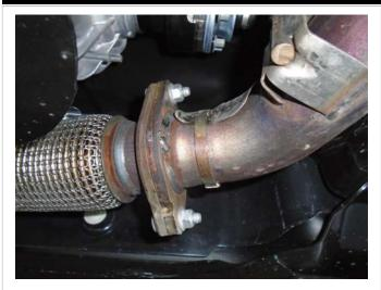
**Step 1:** Begin removal of your OE system by first loosening the fasteners from the front 2 bolt flanges (2) and un-plugging the electrical connections to the valves. Disengage all welded hangers from the rubber insulators. Do not damage the fasteners, heatshields (on the overaxle pipes) and rubber insulators as they will be used to install your new system.
