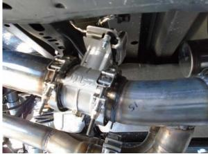
**Step 12:** Next install the valves using the supplied clamps and fit the electrical plugs.
