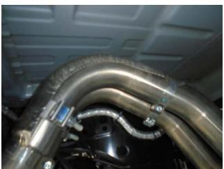
**Step 8:** Before beginning the exhaust installation the heatshields from the OE over axle pipes need to be removed and transferred to the MagnaFlow system. Cut the retaining straps securing the heatshield and move them over to the MagnaFlow Over Axle pipes (2) and secure using the supplied worm drive clamps.
