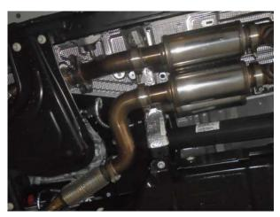
**Step 10:** Loosely install the two Muffler/NDT Resonator Assemblies using the supplied clamps. Orientate as shown
