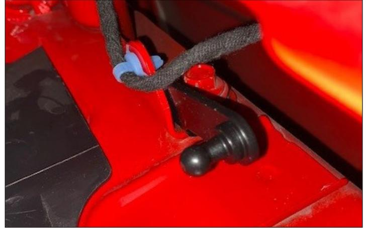
4. Place washer on ball socket stud and start threaded plate. Ensure that 2-3 threads are showing on back side. This will assist in threaded plate retention.
