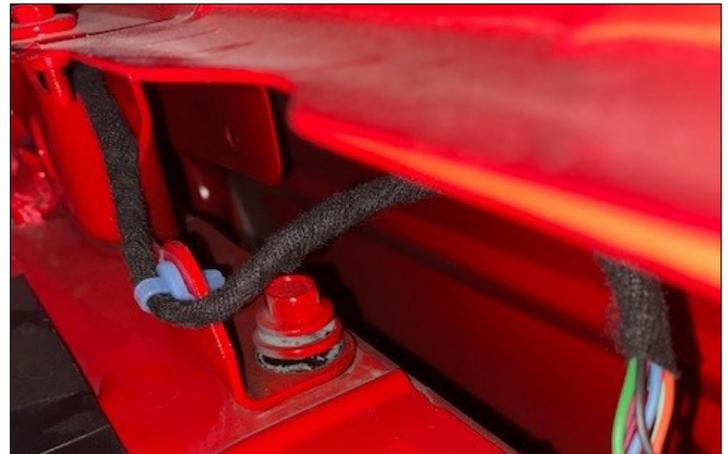
2. Identify Driver Side fender bracket. Ball socket will point towards engine (see image). Install the bolt removed in Step 1.
