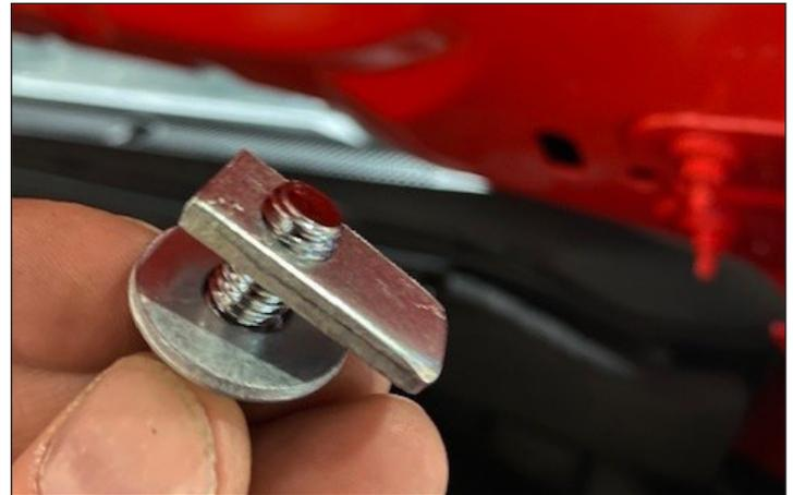
5. Insert threaded plate into hole.
