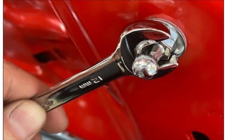
7. Install strut with piston rod pointed down. Install on hood ball socket, then on fender. Repeat steps on passenger side.
