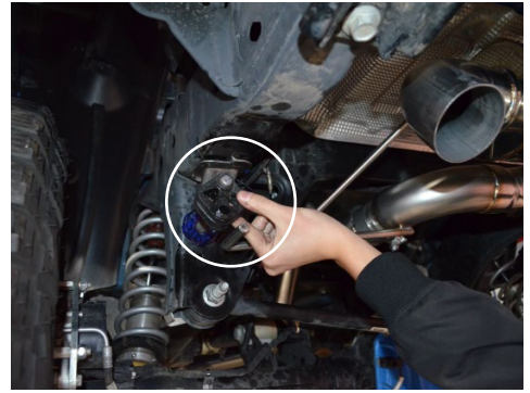
15. Insert the driver side hanger into the rubber insulator.
