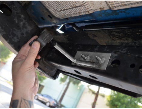
13. 2.3L MODELS ONLY: Insert the rubber insulator onto the exhaust hanger bracket.
