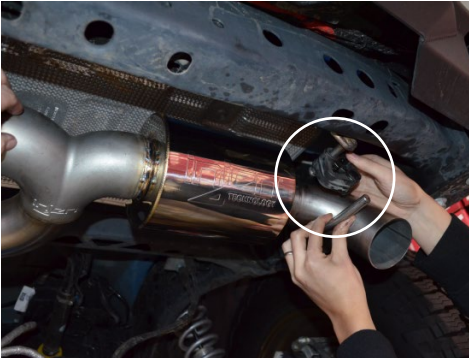
16. Insert the passenger side hanger into the rubber insulator.
