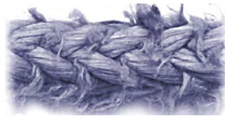
c. Rope must be replaced
